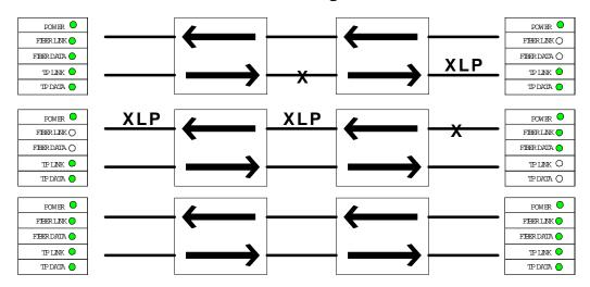
The Diagram above shows the operation of the 3340-3350 10Base Ethernet Links when the Link Pulse option is set to Pass-through mode (Switch marked ONE/FULL set to ONE).
