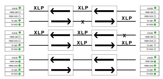
The Diagram above shows the operation of the 3340-3350 10Base Ethernet Links when the Link Pulse option is set to Fail mode(Switch marked ONE/FULL set to FULL).
